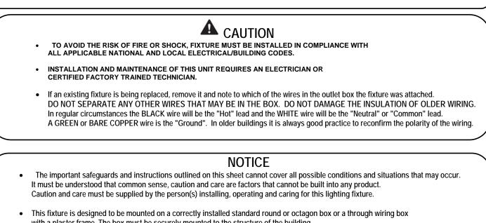
with a plaster frame. The box must be securely mounted to the structure of the building. The crossbar and hardware supplied should be used. Directly mounting the fixture to the outlet box may make it impossible to correctly align the fixture.
