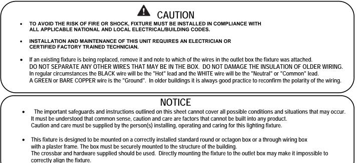
NOTE: For your safety be certain that the circuit breakers controlling outdoor lighting and equipment are GFI breakers
