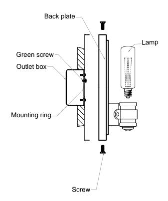
Fasten the white fixture lead to the white wire in the outlet box. Fasten the wires together with an approved fastener (wire nut). Starting about 1" below the fastener, tightly wrap the connection with electrical tape so that the connections seals the end of the fastener.
